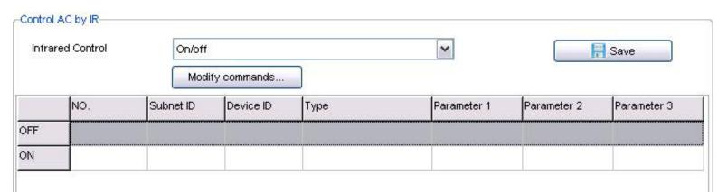
These records will determine what action will happen if the button ON/OFF in the AC page in the DDP is pressed (The first button). In our case we need to tell the IR emitter to send the OFF command when OFF is pressed and ON command when On is pressed.
