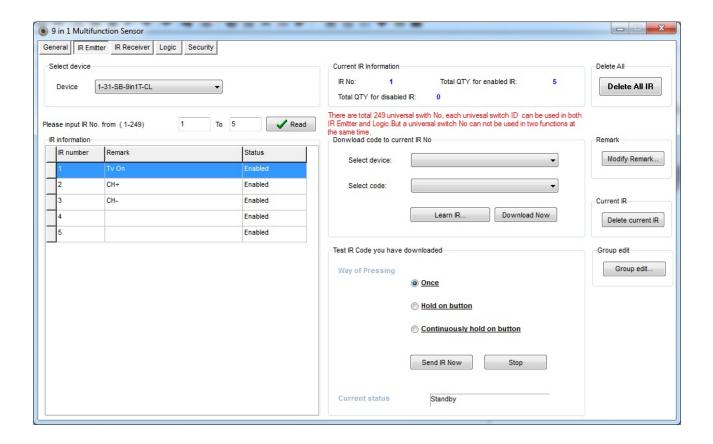
If you want to control any devices has a remote you need first to save its IR codes, For that, connect your IR Learner install the driver (WIN XP):
